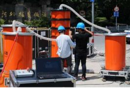
The ohv cable test systems can be designed to meet the specific maximum test voltage as per request. The test system comes in rugged and robust transportation and storage cases which are easy to ship by train, truck or even airplane to the cable test site.
