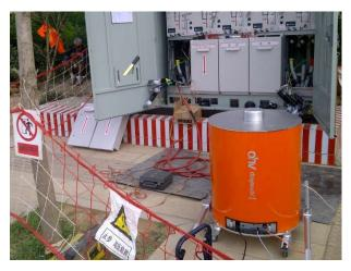
The test system comes in rugged and robust transportation and storage cases which are easy to ship by train, truck or even airplane to the cable test site. All required low and high voltage cables, connectors, calibrator and base load capacitor for testing of short cables are included in the kit.
