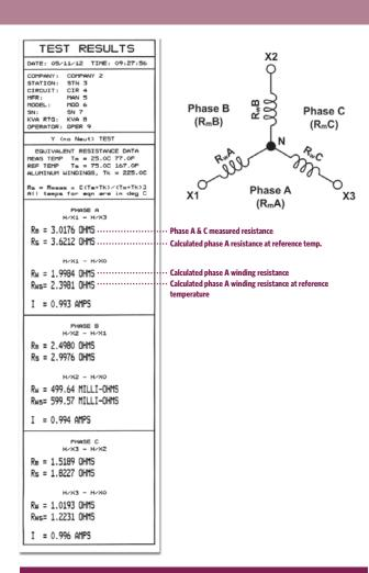
Sample test results showing individual winding resistance values for a Wye transformer with no accessible neutral. The TRM-203/403 can also calculate the phase resistance and individual winding resistance values at a given reference temperature (Rs and Rws, respectively).
