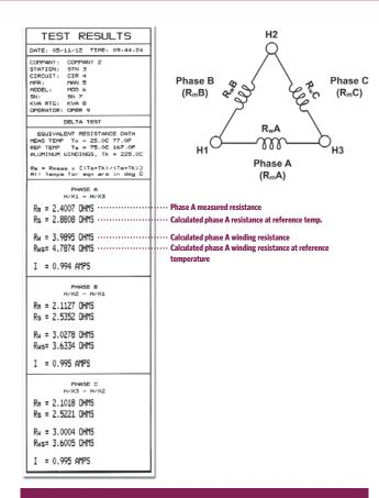
Sample test results showing individual winding resistance values for a Delta transformer. The TRM-203/403 can also calculate the phase resistance and individual winding resistance values at a given reference temperature (Rs and Rws, respectively).
